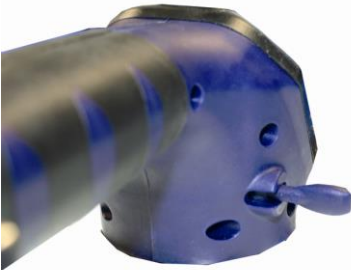
Fig. 19: Lever in horizontal position - working position
