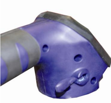
Fig. 18: Lever in vertical position - transport lock
