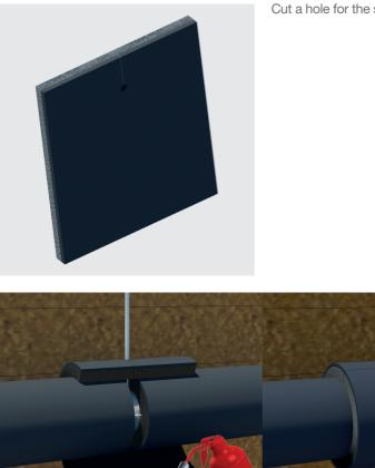
Cut a hole for the screw and apply adhesive.
