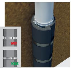
While fixing mechanicaly, use metallic wire, adhesive tape or nylon strips (approx 6 fixing per meter).
